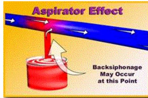
A **cross connection** is any actual or potential physical connection between a potable water line and any pipe, vessel, or machine containing a non potable fluid, or has the possibility of containing a non potable fluid, solid or gas, such that it is possible for the non potable fluid, solid or gas to enter the potable water system by backflow.
